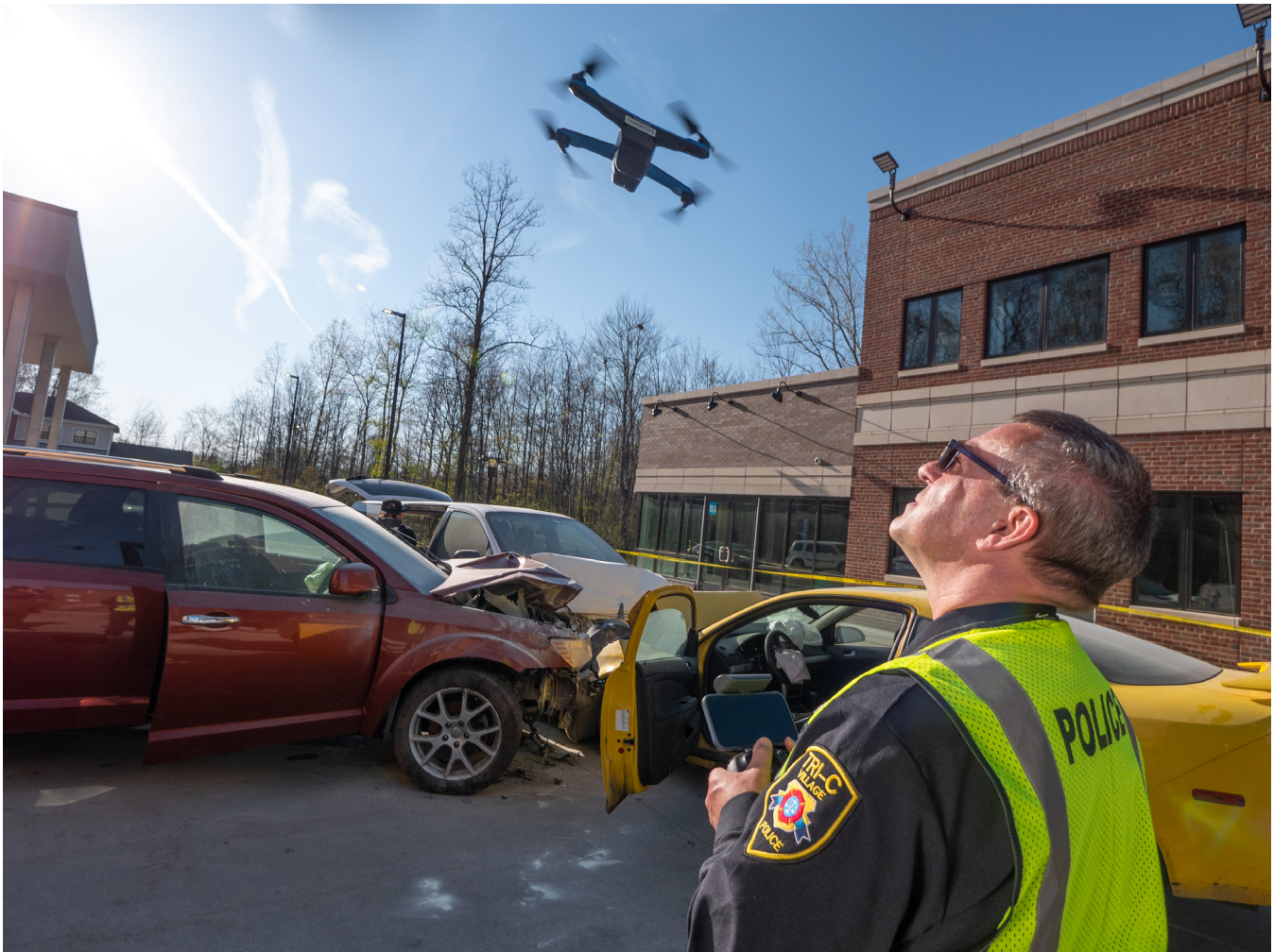
An officer can quickly deploy the Skydio 2 to produce a 3D model of the crash scene with a level of precision that can be attained of all areas of the accident, including the exact orientation and crumple zone of the vehicles. Source: Skydio.
