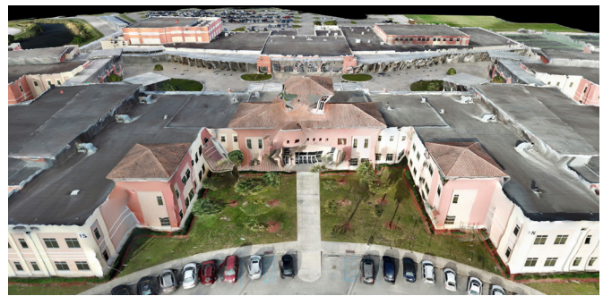
DJI: By comparison, the same flight pattern with DJI generated inaccurate geometry, poor colorization, and inconsistent exposure.
